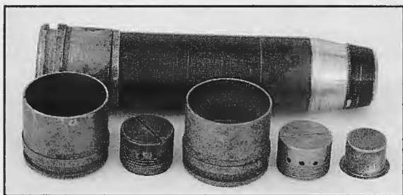
Background: VOG-26 30x28mm grenade — note copper driving band near base of grenade body and blue color code on fuze tip which distinguishes this grenade from VOG-17. Foreground: left to right — fired case with high-pressure chamber removed, unfired case with high-pressure chamber and brass propellant cup.
